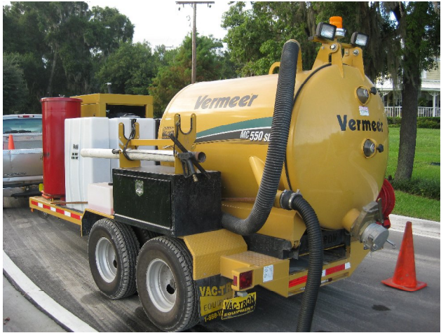
a. Portable Vacuum Unit with 550-Gallon Capacity
